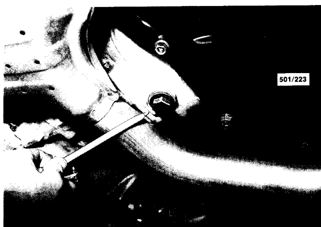
Location of the manual transaxle drain plug, 1986 model shown.
