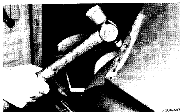
Using a ball peen hammer to tap down the rust affected area.
