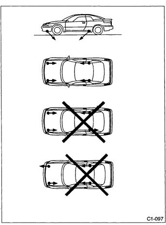
a. Avoid towing another car with front towing hooks.b. Do not tow a vehicle which is heavier than towing vehicle.
