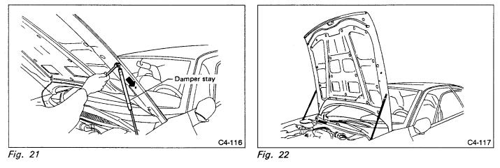
a. If front hood must be opened fully for ease of operation, change the mounting position of the front hood stay.
