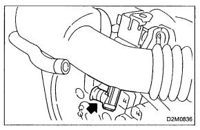
11) Using suitable tape, block the air by-pass hose connection of the air intake boot.
