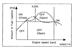
• The induction control valve operates on the intake manifold pressure transmitted to the diaphragm. The intake manifold pressure is controlled by opening/closing the induction control solenoid valve which is determined by the ECM according to the engine speed and amount of fuel injection.
