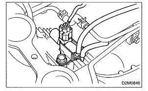
5) Measure resistance of harness between auxiliary air control valve connector and engine ground.
