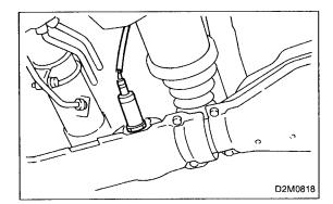
4) Remove front oxygen sensor 1.
