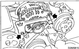
4) Remove bolts which install generator to bracket, then remove generator.
