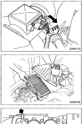
7) Slide connector cover out from mass air flow sensor connector.
