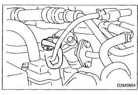
6) Disconnect connectors from each fuel injector.
