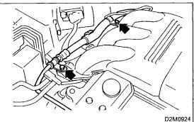
15) Remove bolts which install power steering hose bracket to collector chamber, then position the hose away from collector chamber.
