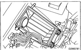
8) Remove air cleaner lower case.9) Installation is in the reverse order of removal.
