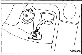
3) Pull out the remote control rearview mirror switch, and disconnect connector from it.
