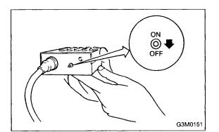
3) Turn ignition switch and select monitor switch to OFF.
