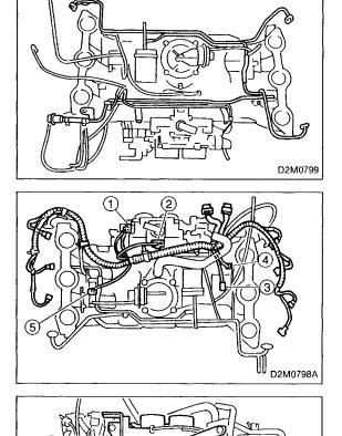
3) Install fuel pipes to collector chamber.
