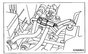
8) Connect power steering switch connector.
