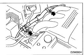
5) Remove bolts which install power steering hose bracket to collector chamber, then position the hose away from collector chamber.
