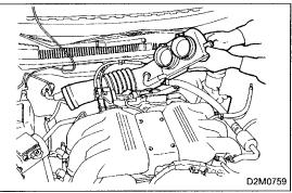
3) Loosen clamps which connect air intake duct to throttle body and mass air flow sensor.
