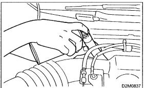
12) While operating the engine in the 1,500 — 2,000 rpm range, spray the cleaner from the air by-pass hose on the idle air control valve for 10 seconds.
