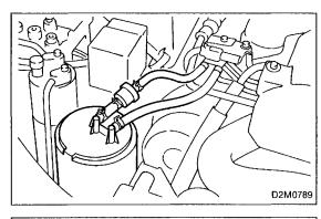
13) Disconnect canister hoses from evaporation pipes.
