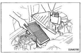
6) Remove clips on air cleaner upper cover.7) Remove air cleaner element.
