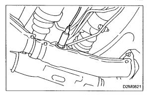
4) Remove front oxygen sensor 2.
