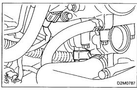
8) Disconnect connectors from throttle position sensor and idle air control solenoid valve.
