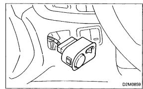
4) Remove bolts which install lower cover panel.5) Lower the panel.
