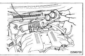
2) Loosen clamps which connect air intake duct to throttle body and mass air flow sensor.
