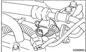
7) Remove screws which hold fuel injector to fuel injector pipe.
