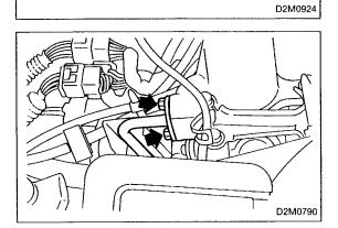
15) Remove EGR pipe cover, then remove bolts which install EGR pipe to collector chamber.
