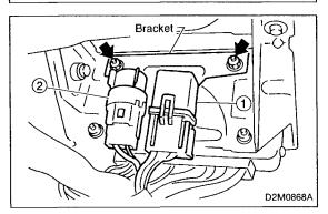
11) Remove nuts which hold the bracket of main relay (1) and fuel pump relay (2).
