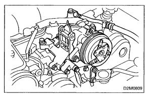
27) Remove A/C compressor with bracket, and move A/C compressor forward to facilitate removal of intake manifold mounting bolts.
