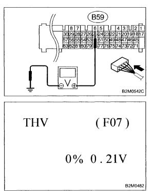
2) Measure voltage between ECM connector and chassis ground.
