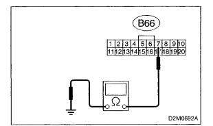
3) Measure resistance of harness between TCM and chassis ground.
