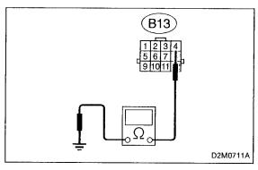
5) Measure resistance of harness between transmission harness connector and transmission ground.
