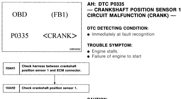
CAUTION: After repair or replacement of faulty parts, conduct CLEAR MEMORY and INSPECTION MODES. < Ref. to 2-7b [T3D0] and [T3E0]. $\Rightarrow$ 5>
