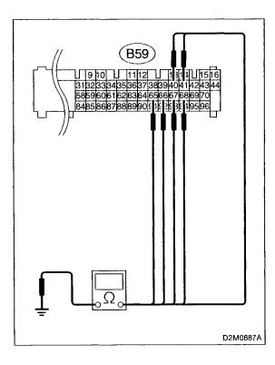
4) Measure resistance of harness between ECM and chassis ground.
