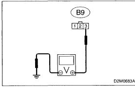
Measure resistance of harness between ECM connector and chassis ground.
