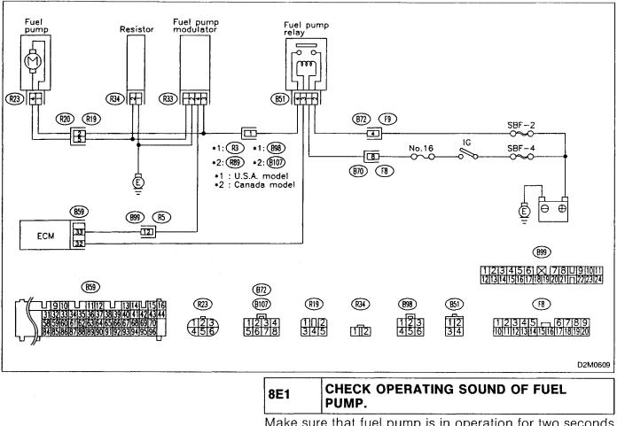
Make sure that fuel pump is in operation for two seconds when turning ignition switch to ON.
