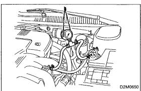
4) Start the engine and idle while gear position is neutral.5) Measure fuel pressure while disconnecting pressure regulator vacuum hose from intake manifold.
