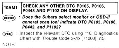
In this case, it is not necessary to inspect DTC P0441.
