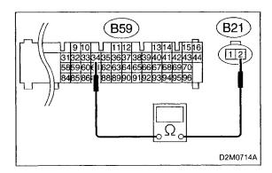
4) Measure resistance of harness between ECM and pressure sources switching solenoid valve connector.
