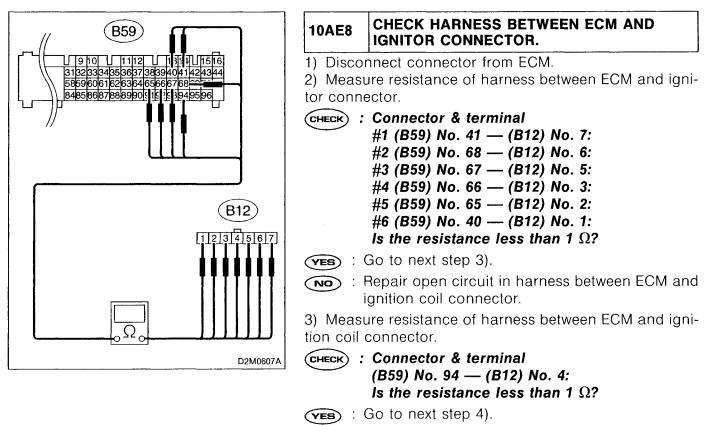
: Repair open circuit in harness between ECM and NO ignition coil connector.
