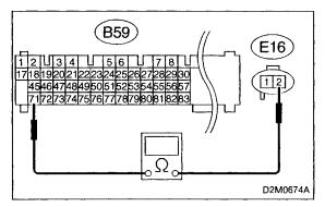
5) Measure resistance of harness between ECM and EGR control solenoid valve connector.
