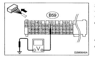
3) Disconnect connector from front oxygen sensor 2 (LH). 4) Measure voltage between ECM connector and chassis ground.
