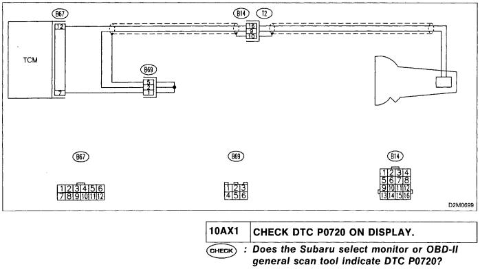
**VES** : Check vehicle speed sensor 1 circuit.
