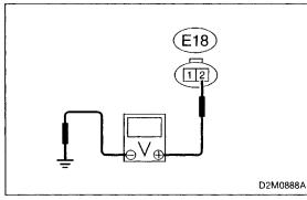
(E18) No. 2 (+) — Engine ground (-): Is the voltage more than 10 V?
