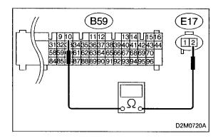
4) Measure resistance of harness between ECM and purge control solenoid valve of harness connector.
