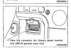
> (2) Open the cover and connect Subaru select monitor to data link connector located in the lower portion of the instrument panel (on the driver's side), to the lower cover.
