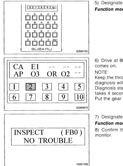
5) Designate mode using function key. Function mode: FA4
