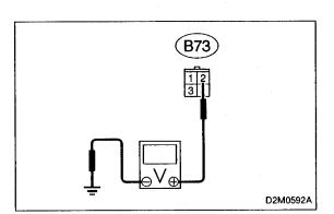
4) Measure voltage between starter interrupt relay connector and chassis ground.
