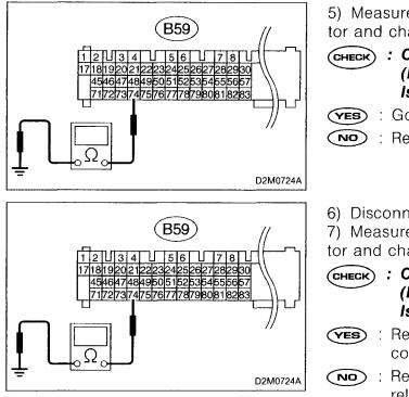
5) Measure resistance of harness between ECM connector and chassis ground.
