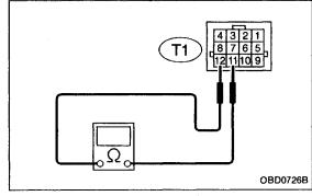
6) Measure power supply voltage between ignition switch connector and chassis ground.
