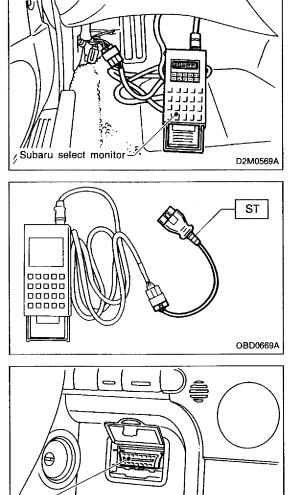
6) Connect Subaru select monitor to data link connector.
