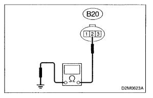
8) Measure resistance of harness between pressure sensor connector and engine ground.
