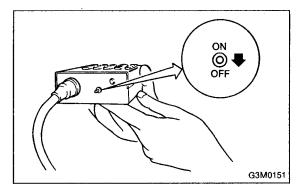
6) After the display is gone, turn Subaru select monitor switch and ignition switch to OFF.
