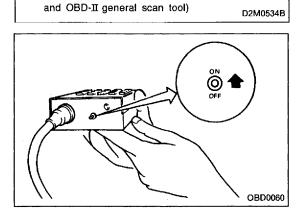
Data link connector (for Subaru select monitor
