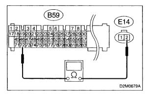
5) Measure resistance of harness between ECM and purge control solenoid valve of harness connector.
