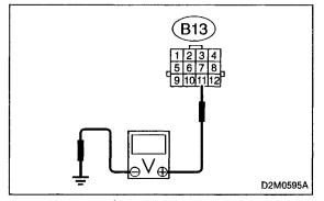
11) Measure voltage between transmission harness connector and transmission ground.
