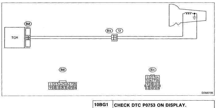
CHECK : Does the Subaru select monitor or OBD-II general scan tool indicate DTC P0753?
