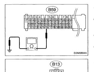
4) Measure resistance of harness between ECM and chassis ground.
