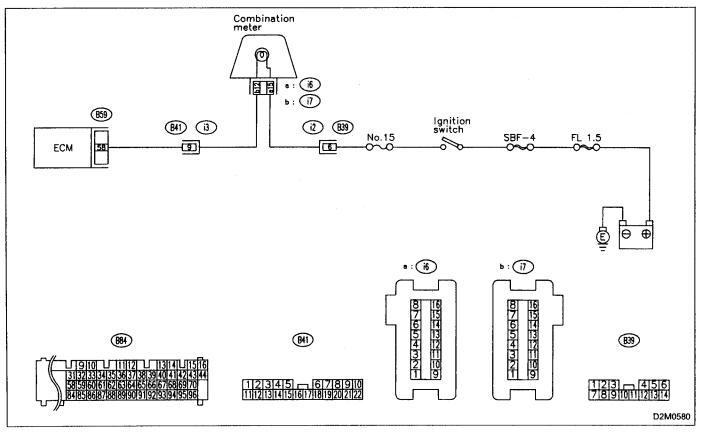
7. Diagnostics for CHECK ENGINE Malfunction Indicator Lamp (MIL)
