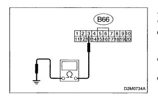
4) Measure resistance of harness between TCM and chassis ground.
