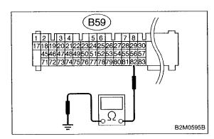
4) Measure resistance of harness between ECM and chassis ground.
