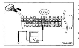
3) Disconnect connector from rear oxygen sensor.
