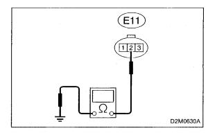
8) Measure resistance of harness between throttle position sensor connector and engine ground.
