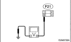
3) Measure voltage between fuse connector and engine ground.
