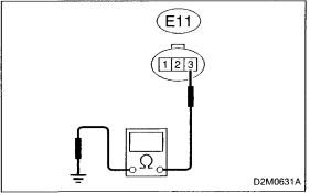
4) Measure resistance of harness between throttle position sensor connector and engine ground.
