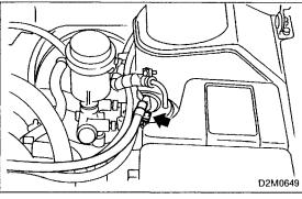
3) Disconnect fuel delivery hose from fuel filter, and connect fuel pressure gauge.
