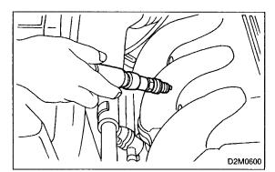
3) Disconnect connector from ignition coil on normal cylinder and remove normal ignition coil.
