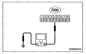
10) Measure voltage between security electronic module connector and chassis ground.
