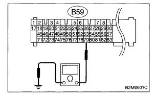
4) Measure resistance of harness between ECM connector and chassis ground.
