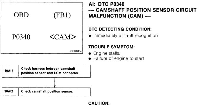
After repair or replacement of faulty parts, conduct CLEAR MEMORY and INSPECTION MODES. <Ref. to 2-7b [T3D0] and [T3E0].☆5>
