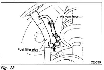
Place a container under pipe connection to catch fuel which way remain in filler pipe.
