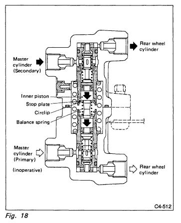
2) As the master cylinder fluid pressure increases, it overcomes spring tension. This causes the secondary valve piston and inner piston to move toward the primary circuit as a unit. The valve is held open since it is pulled by the inner piston connector. For this reason, the fluid pressure in the secondary circuit of the rear wheel cylinder is not controlled as it decreases.
