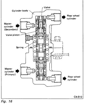
3) As master cylinder fluid pressure increases further, the valve piston moves further outward. The valve then comes in contact with the cylinder body so that the valve is opened.
