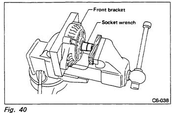
(3) Set a new bearing and closely install a fit jig on the bearing outer race. Press the bearing down into place with a hand press or vise. A socket wrench can serve as the jig.
