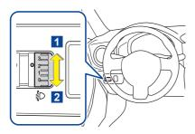
The level of the headlights can be adjusted according to the number of passengers and the loading condition of the vehicle.
