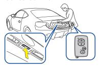
Carry the access key, and press the button to unlock the trunk lid.
