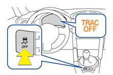
To turn the Traction Control System off, quickly press and release the button.
