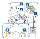
Each time the select lever or paddle shift levers are operated, the gear changes up or down one gear and the selected gear, 1 through 6, will be set. The selected gear, from 1 to 6, and M will be displayed on the shift position and shift range indicator.
