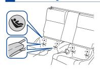
LATCH anchors are provided for both rear seats. (Buttons displaying the location of the anchors are attached to the seats.) See the Owner's Manual Chapter 1 for details.
