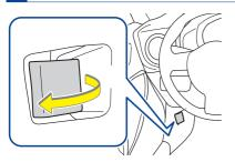
Pull the engine hood release lever. The engine hood will pop up slightly.
