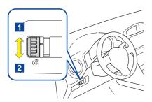
The brightness of the instrument panel lights can be adjusted.
