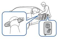
Carry the access key, and grip the driver's door handle to unlock the door.
