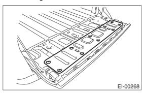
3) Remove rod clamp. Remove nuts and detach lock handle.
