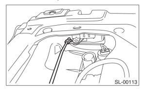
4) Remove bolts and tail gate latch.
