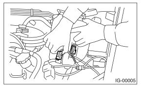
3) Disconnect the rear window glass washer hose from washer motor, then plug connection with a suitable cap.
