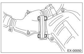
2) Install front and center exhaust pipe assembly to the vehicle.
