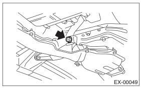
4) Tighten nuts which hold front exhaust pipe onto cylinder heads.
