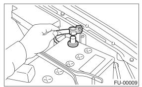
2) Disconnect front oxygen (A/F) sensor connector.
