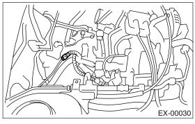
10) Connect front oxygen (A/F) sensor connector.
