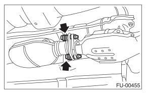
2) Separate rear exhaust pipe from muffler.
