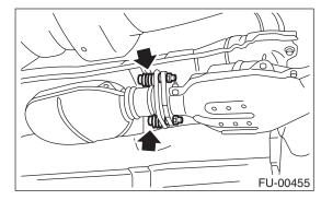
7) Tighten bolt which holds front and center exhaust pipe assembly to hanger bracket.
