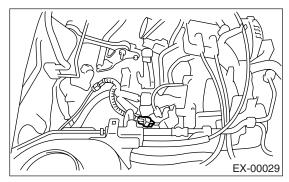
3) Disconnect rear oxygen sensor connector.
