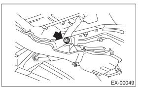
9) Remove front and center exhaust pipe assembly from the vehicle.
