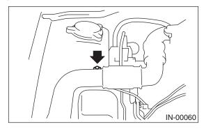
3) Remove air intake ducts as a unit.
