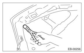
3) Remove the bolts to disconnect the hood from hinges.
