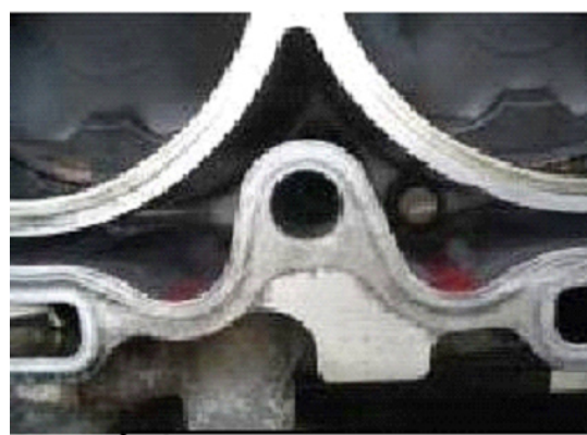
After cleaning coolant sealing portion (block)
