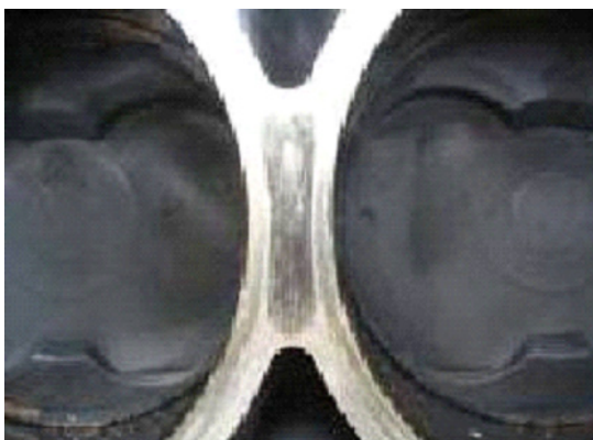
After cleaning bore sealing portion (block)
