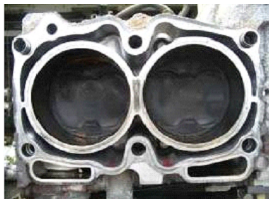
Finished cleaning (block)
