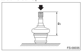
(2) While applying 686 N (70 kgf, 154 lb) of force in the direction shown in the figure, measure dimension  $\,\varrho_{\,2}.\,$
