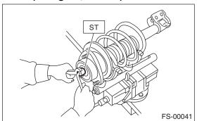
10) Loosen the coil spring carefully.
