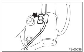
5) Remove the two bolts securing the housing to the strut.
