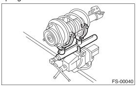
2) Using the ST, remove the self-locking nut. ST 927760000 STRUT MOUNT SOCKET
