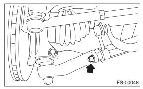
5) Remove the bolt and nut which secures the stabilizer to the crossmember.
