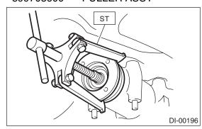
12) Using the ST, remove the oil seal. ST 398527700 PULLER ASSY
