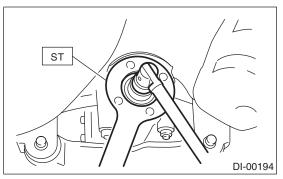
11) Extract the companion flange using ST. ST 399703600 PULLER ASSY
