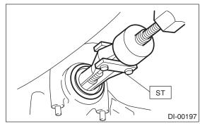
13) Install a new oil seal using ST.
