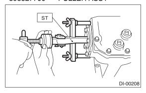
9) Install a new side oil seal using the ST.
