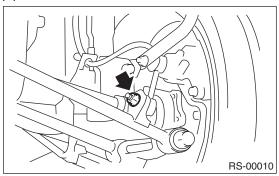
(5) Remove the bolts which secure the trailing link to the housing.
