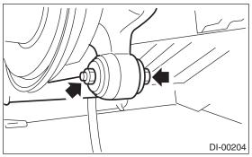
(6) Remove the bolts which secure the front and rear lateral links to the rear housing.
