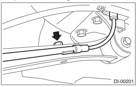
(3) Remove the ABS wheel speed sensor cable clamp and the parking brake cable guide from the trailing link.
