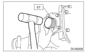
10) Insert the DOJ into rear differential.(1) Attach the ST to rear differential.ST 28099PA090 SIDE OIL SEAL PROTECTOR
