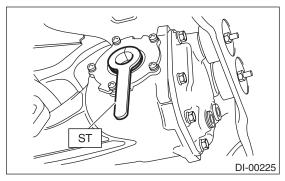
(2) Install the spline shaft until the spline portion is inside the side oil seal using ST.
