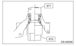
7) Using the ST1 and ST2, press the inner oil seal until it contacts the circlip.
