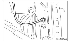
10) Remove the transverse link ball joint from the housing.
