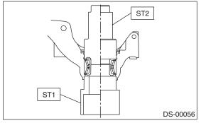
5) Using a pliers, securely install the snap ring.
