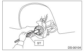
12) While pressing the brake pedal, tighten a new axle nut to the specified torque.
