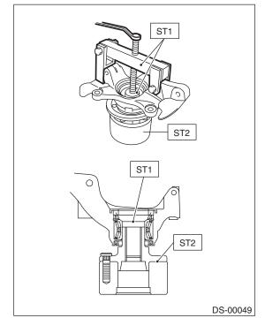
If inner bearing race remains in the hub, remove it with a suitable tool (commercially available tools).
