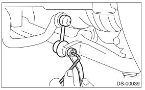
5) Remove the disc brake caliper from the housing, and suspend it from strut using a wire.
