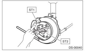
13) After scribing an alignment mark on the camber adjusting bolt head, remove bolts connecting the housing and strut, and disconnect the housing from the strut.
