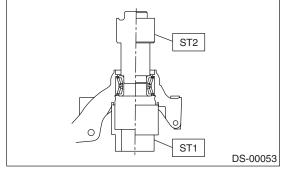
8) Using the ST and a hydraulic press, push out the hub bolts.
