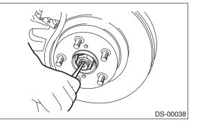
3) Remove the axle nut using a socket wrench while depressing the brake pedal.
