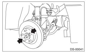
7) Remove the cotter pin and castle nut securing the tie-rod end to the housing knuckle arm.
