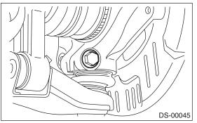
11) Remove the front drive shaft assembly from the hub. If it is hard to remove, use the STs.
