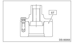
2) Using a press, press the new hub bolts until their seating surfaces contact the hub.
