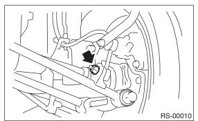
3) Remove the bolt which secures the stabilizer to the stabilizer bracket.
