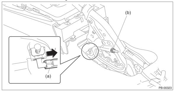
(3) Remove the bolt, and then remove the lever assembly - hand brake.
