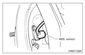
15) Remove bolts which secure rear housing to strut, and separate the two.
