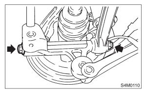
12) Disengage BJ from housing splines, and remove rear drive shaft assembly. If it is hard to remove, use STs.
