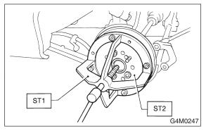
13) Remove rear ABS sensor from back plate (only vehicle equipped with ABS).
