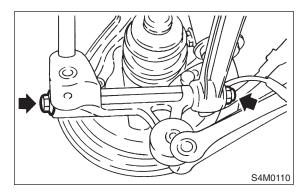
13) Disengage BJ from housing splines, and remove rear drive shaft assembly. If it is hard to remove, use STs.
