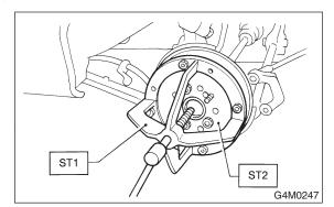
14) Remove rear ABS sensor from back plate (only vehicle equipped with ABS).
