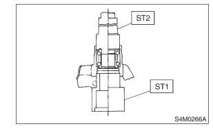
4) Using plier, install snap ring.
