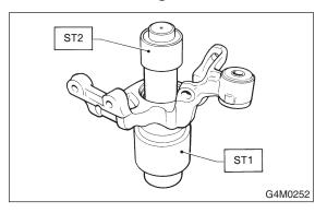
6) Remove tone wheel bolts and remove tone wheel from hub (only vehicle equipped with ABS).7) Using ST, press hub bolt out.
