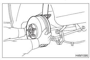
9) Connect rear housing assembly to trailing link assembly, and tighten self-locking nut.
