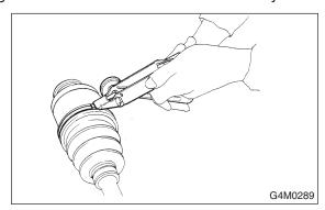
16) Tap on the clip with the punch provided at the end of ST.
