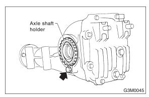
10) Remove axle nut and drive shaft. If it is hard to remove, use ST1 and ST2.
