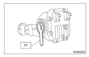
6) Insert DOJ spline end into bore of side oil seal, and remove ST.
