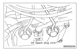
6) Remove spark plug with the spark plug socket.
