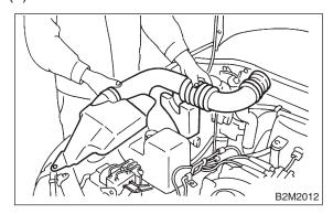
(4) Remove resonator chamber.
