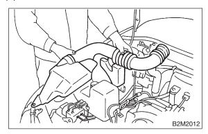
(4) Remove resonator chamber.
