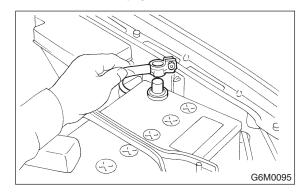
2) Remove air intake duct and resonator chamber.(1) Remove bolt which installs air intake duct
