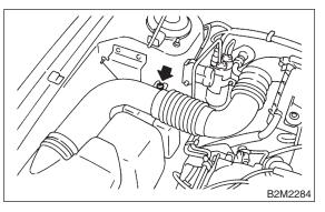
(3) Remove air intake duct as a unit.
