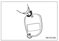
1. Remove the two screws on the back of the transmitter case by using a phillips screwdriver.
