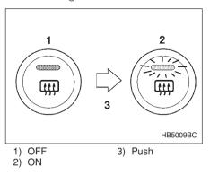
To turn on the defogger, push the switch. To turn it off, push the switch again.
