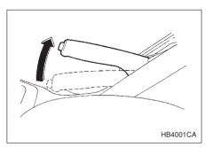
Check the parking brake stroke according to the maintenance schedule in the "Warranty and Maintenance Booklet". When the parking brake is properly adjusted, braking power is fully applied by pulling the lever up seven to eight notches gently but firmly (about 44 lb, 196 N, 20 kg). If the parking brake lever stroke is not within the specified range, have the brake system checked and adjusted at your SUBARU dealer.
