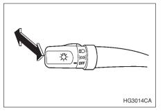
To change from low beam to high beam, push the turn signal lever forward. When the headlights are on high beam, the high beam indicator light " $\equiv O$ " on the instrument panel is also on.
