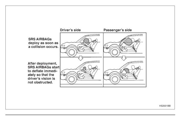
When the SRS airbag deploys, a sudden, fairly loud inflation noise will be heard and some smoke will be released. These occurrences are normal result of the deployment. This smoke does not indicate a fire in the vehicle.
