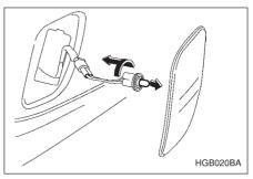
1. Remove the front side marker light assembly by prying the edge of the lens with a regular screwdriver. At this time, use a cloth to protect the body from being damaged by the screwdriver.
