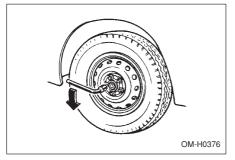
7. Loosen the wheel nuts using the wheel nut wrench but do not remove the nuts.
