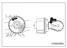
1. Remove the bulb socket from the headlight assembly by turning it counterclockwise.
