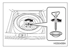
15. Store the flat tire in the spare tire compartment. Put the spacer and tighten the attaching bolt firmly. Also store the jack and wheel nut wrench in their storage locations.
