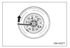
14. Use the wheel nut wrench to securely tighten the wheel nuts to the specified torque, following the tightening order in the illustration.
