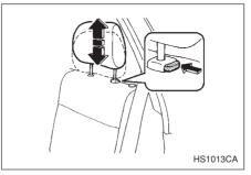
To raise the headrest, pull it up. To lower it, push the head rest down while depressing the release button on the top of the seatback.
