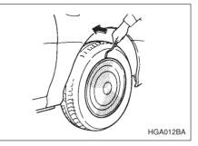
Insert the wheel cover remover into the notch provided, and pry the wheel cover off.
