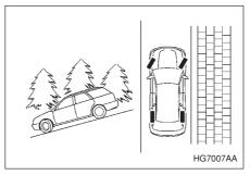
When facing downhill, the front wheels should be turned into the curb.
