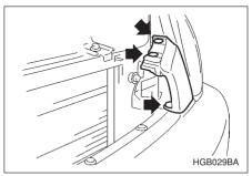
3. Remove three bolts and disconnect connectors, and then detach headlight assembly.
