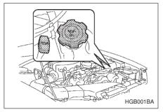
3. Be sure the dipstick is correctly inserted until it stops with the graphic symbol  $\forall r \rightarrow$  on its top appearing as shown in the illustration.
