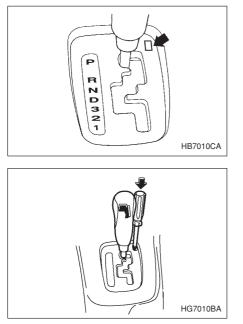
4. Insert the screwdriver into the hole.
