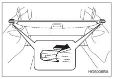
2. Pull either sleeve on the end of the cover housing to shorten the cover's length.
