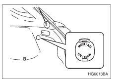
Electrical power (12V DC) from the battery is on tap at the socket when the ignition switch is either in the "ACC" or "ON" position.
