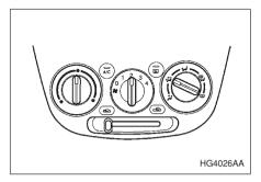
This setting allows you to direct air of different temperatures from the instrument panel and foot outlets. The air from the foot outlets is slightly warmer than from the instrument panel outlets.
