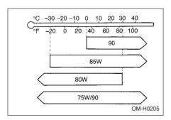
SAE viscosity No. and Applicable Temperature
