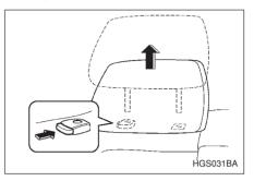
1. Remove the headrest at the seating position where the child restraint system has been installed with the seatbelt or lower anchorages; lift up the headrest while pressing the release button. Store the headrest in the cargo area. Avoid placing the headrest in the passenger compartment to prevent it from being thrown around in the passenger compartment in a sudden stop or a sharp turn.
