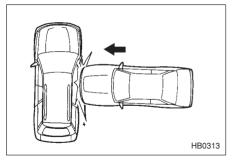
A severe side impact near the front seat activates the SRS side airbag.
