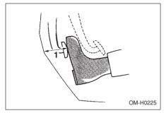
1) Left hand drive vehicles: More than 2.56 in (65 mm) Right hand drive vehicles: More than 3.35 in (85 mm)
