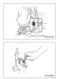
1. Insert a key or other hard pointed object into the slot in the connector (buckle) on the right-hand side and push it in, and the connector (tongue) plate will
