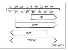
SAE viscosity No. and Applicable Temperature
