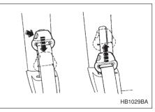
Always adjust the anchor height so that the shoulder belt passes over the middle of the shoulder without touching the neck.
