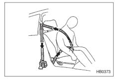
When a seatbelt pretensioner is activated, an operating noise will be heard and a small amount of smoke will be released. These occurrences are normal and not harmful. This smoke does not indicate a fire in the vehicle.
