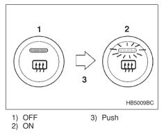
To turn on the outside mirror defogger, push the switch. To turn it off, push the switch again. The indicator light located on the switch lights up while the outside mirror defogger is operating.
