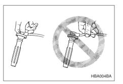
It may be difficult to replace the spark plugs. It is recommended that you have the spark plugs replaced by your SUBARU dealer.
