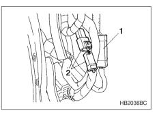
1) Connector for SRS airbag system (yellow)
