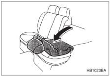
Unlock the seatback by pulling the release knob and then fold the seatback down.
