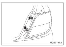
2. Remove the upper and lower screws. Then, slide the rear combination lamp assembly to the rear and remove it from the vehicle.
