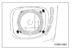
1. Remove the front fog light assembly by removing the three bolts.
