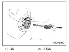
2. Turn the ignition switch from "ON" to "LOCK" position and remove the key from the ignition switch.
