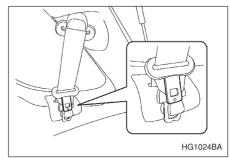
2. Allow the retractor to roll up the belt. You should hold the webbing end and guide it back into the retractor while it is rolling up. Insert the tongue plate into the belt holder.
