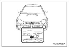
2. Release the secondary hood release located under the front grille by moving the lever toward the left.
