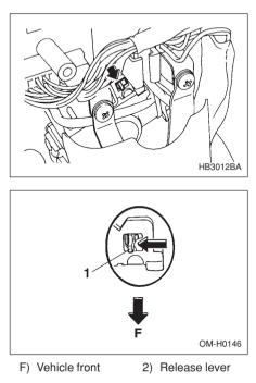
3. Turn the ignition key while pressing the key interlock release lever. Take your vehicle to the nearest SUBARU dealer immediately to have the key interlock system repaired.
