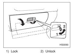
To open the glove compartment, pull the handle. To close it, push the lid firmly upward.
