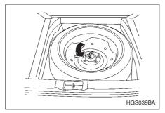
**Sedan:** Remove the floor cover from the trunk. Remove the storage tray (if so equipped). Turn the attaching bolt counterclockwise, then take the spare tire out.
