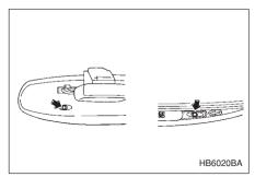
The mirror has a photosensor attached on both the front and back sides. If the glare from the headlights of vehicles behind you strikes the mirror, these sensors detect it and make the reflection surface of the mirror dimmer to help prevent you from being blinded. For this reason, use care not to cover the sensors with stickers, or other similar items. Periodically wipe the sensors clean using a piece of dry soft cotton cloth or an applicator.
