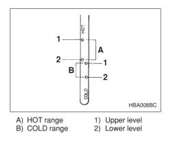
4. Pull out the dipstick and check the fluid level on the gauge. If it is below the lower level on the "HOT" range, add the recommended automatic transmission fluid up to the upper level.
