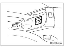
The seat heater operates when the ignition switch is either in the "ACC" or "ON" position.
