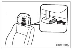
To lower it, push the head restraint down while pressing the release button on the top of the seatback.
