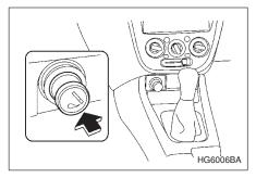
The cigarette lighter operates only when the ignition switch is in the "ON" and "ACC" positions.
