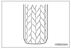
Roadholding is good, and steering is responsive. Rolling resistance is low, so fuel consumption is also lower. • Abnormally low tire pressure (tread worn at shoulders)
