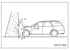
A head-on collision against a thick concrete wall at a vehicle speed of 12 to 19 mph (20 to 30 km/h) activates the SRS frontal airbag. The SRS frontal airbag will also be activated when the vehicle is exposed to a frontal impact similar in fashion and magnitude to the above-mentioned collision.
