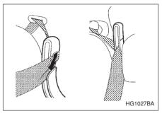
2. After drawing out the seatbelt, pass it through the belt guide as follows: First insert one edge of the belt into the open gap in the comfort guide; then slide the rest of the belt in, so that the whole belt fits inside.
