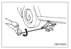
Insert the jack handle into the jackscrew, and turn the handle until the tire clears the ground. Do not raise the vehicle higher than necessary.
