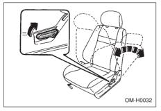
Pull the reclining lever up and adjust the seatback to the desired position. Then release the lever and make sure the seatback is securely locked into place.
