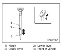
4. Pull out the dipstick again and check the oil level on it. If it is below the lower level, add oil to bring the level up to the upper level.
