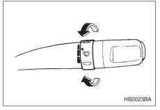
When the wiper switch is in the "To position, turn the dial to adjust the operating interval of the wiper.
