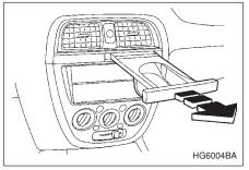
To use the cup holder, push its front surface and pull it out completely.
