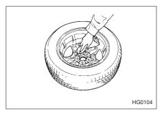
11. Before putting the spare tire on, clean the mounting surface of the wheel and hub with a cloth.12. Put on the spare tire. Replace the wheel nuts. Tighten them by hand.
