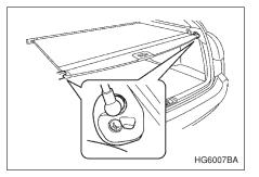
To extend the cover, pull the end of the cover out of the housing, then insert its hooks into the catches as shown. To rewind it, unhook it from the catches and it will rewind automatically. You should hold on to the cover and guide it back into the cover housing while it is rewinding.
