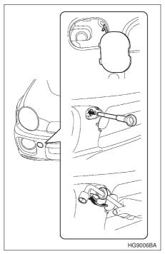
1. Take out the towing eye, screwdriver and wheel nut wrench from the on board tool bag.
