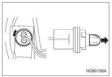
Pull the bulb out of the socket. Install a new bulb.
