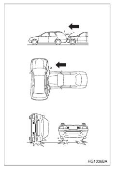
The SRS frontal airbag is basically not designed to deploy if the vehicle is struck from side or from behind, or if it rolls onto its side or roof, or if it is involved in a low-speed frontal collision.
