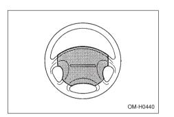
To sound the horn, push the horn pad.
