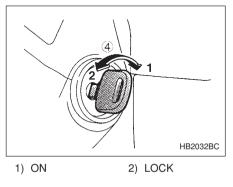
4. Place the ignition key into the ignition switch and cycle the switch from LOCK to ON ten times **within 15 seconds**. Be sure to stop at the LOCK position. The horn will sound once to indicate that you are in the transmitter programming mode.
