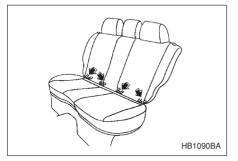
The lower anchorages (bars) are used for installing a child restraint system only on the rear seat window-side seating positions. For each window-side seating position, two lower anchorages are provided.
