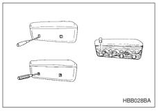
1. Remove the mounting screw covers by prying the edge with a screwdriver.
