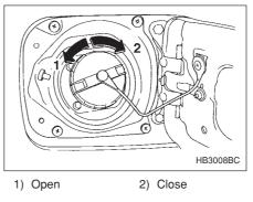
2. Remove the fuel filler cap by turning it slowly counterclockwise.
