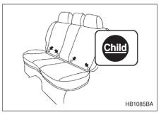
You will find marks "Child" at the bottom of the rear seat seatbacks. These marks indicate the positions of the lower anchorages (bars).
