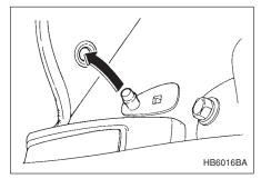
The floor mat is secured using the built-in grommet, by placing the grommet over the pin and pushing downward.
