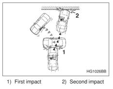
Example: In the case of a double collision, first with another vehicle, then against a concrete wall in immediate succession, the SRS frontal airbag is activated on the first impact but not on the second.
