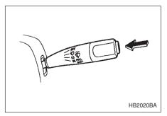
To wash the windshield, push the washer button at the end of the wiper control lever. The washer fluid sprays until you release the washer button. The wipers operate while you push the button.
