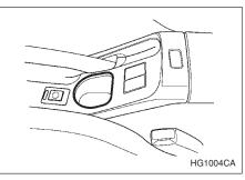
The front passenger's cup holder is built in the center console, beside the parking brake lever.
