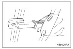
5. Use only a hitch ball that is appropriate for the ball mount and your trailer. The hitch ball must be securely installed on the ball mount.
