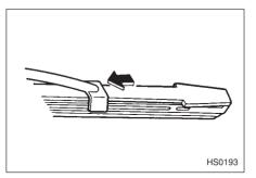
5. Align the claws of the metal support with the grooves in the rubber and slide the blade rubber assembly into the metal support until it locks.
