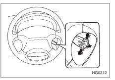
3. Push the control lever downward in the "SET, COAST" direction and release it. Then release the accelerator pedal.
