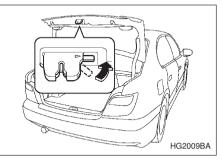
The inside trunk lid release can be cancelled to help prevent unauthorized entry into the trunk. To cancel the trunk lid release, set the lid release cancel lever (located on the inside of the trunk lid, mounted to the trunk lid latch) to the "CANCEL" position. When this lock is in the "CANCEL" position, the trunk can be opened only with the key.
