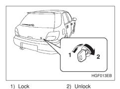
To unlock the rear gate, insert the key in the keyhole and turn it clockwise. To lock the rear gate, insert the key in the keyhole and turn it counterclockwise. If your vehicle is equipped with power door locking switches, the rear gate can also be locked and unlocked through use of the power door locking switches. Refer to the "Power door locking switches" section in this chapter.
