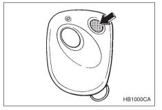
1. Press "UNLOCK/DISARM" button to disarm the security system. (If your vehicle is equipped with the optional security system.)
