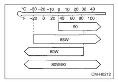
SAE viscosity No. and Applicable Temperature
