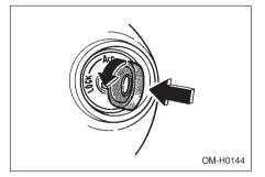
The key can be turned from "ACC" to "LOCK" only when the key is pushed in while turning it.
