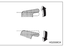
To open the passengers' windows, push the appropriate switch down and hold it until the window reaches the desired position. To close the window, pull the switch up and hold it until it reaches the desired position.
