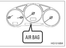
A diagnostic system continually monitors the readiness of the seatbelt pretensioner while the vehicle is being driven. The seatbelt pretensioners share the control module with the SRS airbag system. Therefore, if any malfunction occurs in a seatbelt pretensioner, the SRS airbag system warning light will illuminate. The SRS airbag system warning light will show normal system operation by lighting for about 6 seconds when the ignition key is turned to the "ON" position.
