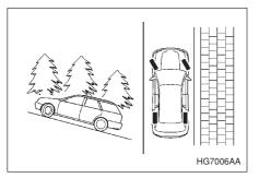
When parking on a hill, always turn the steering wheel. When the vehicle is headed up the hill, the
