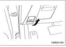
1. Pull the hood release knob under the instrument panel.
