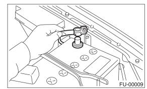
2) Disconnect the washer motor connector.
