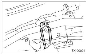
2) Apply a coat of SUBARU CRC to the mating area of cushion rubbers in advance.
