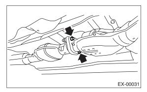
6) Remove the under cover.7) Remove the nuts which hold the front exhaust pipe onto cylinder heads.
