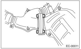
3) Install the front and center exhaust pipe assembly to vehicle.
