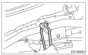
3) Apply a coat of SUBARU CRC to the mating area of cushion rubbers in advance.
