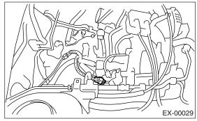
3) Disconnect the rear oxygen sensor connector.
