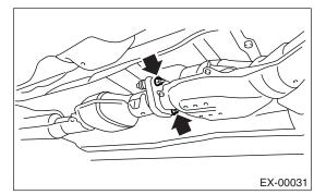
8) Tighten the bolt which holds the front and center exhaust pipe assembly to hanger bracket.
