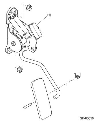
(1) Accelerator pedal position sensor
