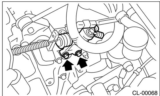
2) Fix the piston with clamp to avoid the piston from jumping out.
