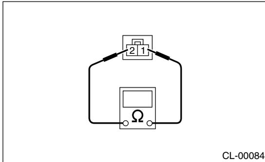
Clutch switch (Starter interlock)
