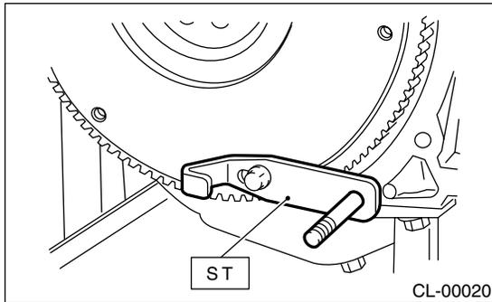
2) Tighten the flywheel attaching bolts to the specified torque.
