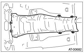
9) Remove the stay from transmission bracket.
