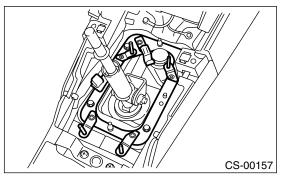
10) Install console box. <Ref. to EI-43, INSTALLA-TION, Console Box.>
