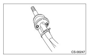
6) Fix the slider and reverse check cable end with spring pin.
