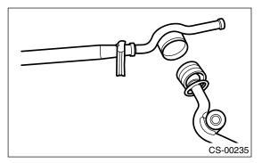
6) Install the washer and snap ring.
