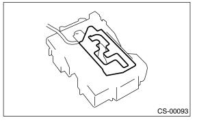
10) Remove the clip, and then remove the "P" range switch.
