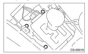
3) Install the console box. <Ref. to EI-43, INSTAL-LATION, Console Box.>
