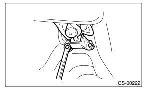
Move the transmission to right side, and then install the joint COMPL and stay.
