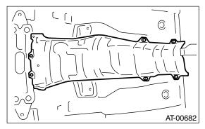
8) Install the rear exhaust pipe and muffler. SOHC model
