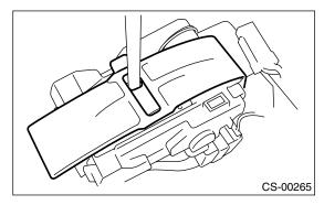
R VOCONTROL SYSTEMS 6) Remove the clip, and then remove the guide udios plate.
