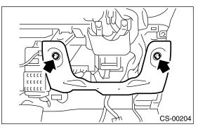
4) Disconnect the connector from body integrated unit.
