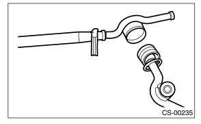
13) Remove the boot and bush from gear shift lever.
