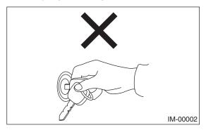
• When repeatedly turning the ignition switch to ON or OFF while diagnostic items are being checked, it should be switched in cycles of "ON" for at least 5 seconds  $\rightarrow$  "OFF" for at least 8 seconds.
