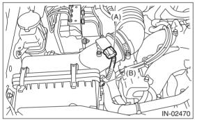
3) Loosen the clamp (A) which connects the air cleaner case to intake boot.
