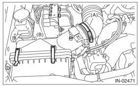
5) Remove the air cleaner case (rear) and air cleaner element.
