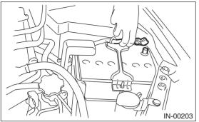
2) Disconnect the connector (A) from the mass air flow and intake air temperature sensor, and remove the clip (B).
