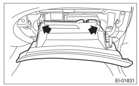
3) Pinch the claw to unlock and remove the A/C filter.
