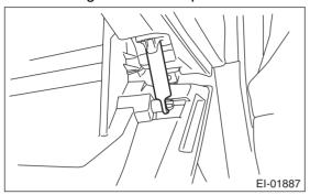
2) Disengage the stopper section and pull the glove box lid to remove it.
