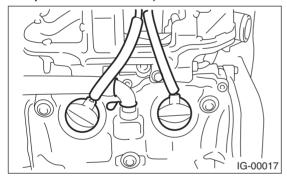
4) Remove the spark plug with a spark plug socket.
