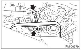
8) Start and run the engine for approximately five minutes to allow the V-belt to become fitted. (When using the gauge)
