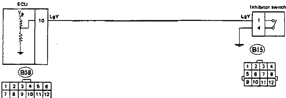
Fig. 40: Schematic - Code 51, Inhibitor Switch (Auto. Trans.)
