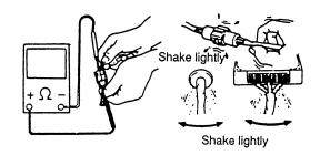
• Lightly shake the connector and the harness, and check for sudden changes in voltage or resistance.
