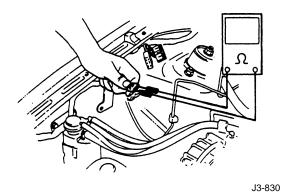
• Checking the connection (range set to  $\Omega$ )
