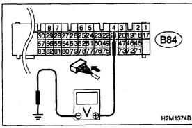
2) Measure voltage between ECM and chassis ground.
