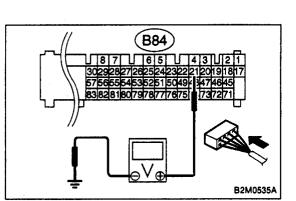
(CHECK): Does the voltage change more than 4.5 V by shaking harness and connector of ECM while monitoring the value with voltage meter?
