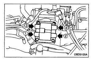
2) Measure resistance between spark plug cord contact portions to check secondary coil.
