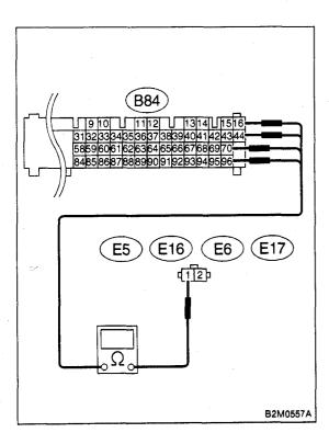
4) Measure resistance of harness connector between ECM connector and fuel injector on faulty cylinders.
