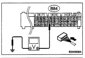
Measure voltage between ECM and chassis ground.
