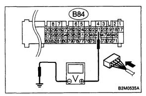
: Does the voltage change more than 4.5 V by shaking harness and connector of ECM while monitoring the value with voltage meter?
