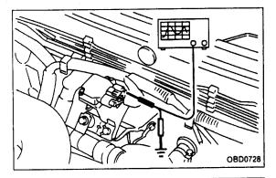
8D5 CHECK INPUT SIGNAL FOR IGNITOR.
