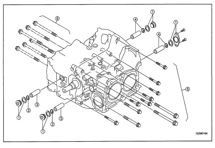
1) Remove service hole cover and service hole plugs using hexagon wrench (14 mm).
