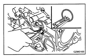
2) Rotate crankshaft to bring #1 and #2 pistons to bottom dead center position, then remove piston circlip through service hole of #1 and #2 cylinders.
