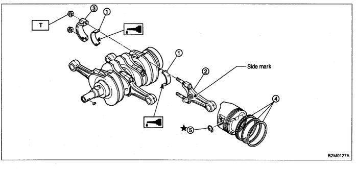
Tightening torque: N·m (kg-m, ft-lb) T: 44±2 (4.5±0.2, 32.5±1.4)
