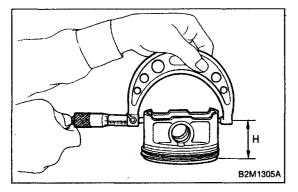
4) How to measure the outer diameter of each piston Measure the outer diameter of each piston at the height shown in the Figure. (Thrust direction)
