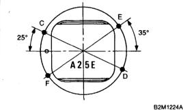
4) Installation of piston rings and oil ring
