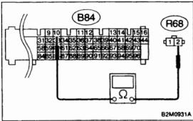
4) Measure resistance of harness between ECM and fuel tank pressure control solenoid valve connector.
