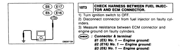
Is the resistance less than 10  $\Omega$ ? (VEB) : Repair short circuit in harness between fuel injector and ECM connector.
