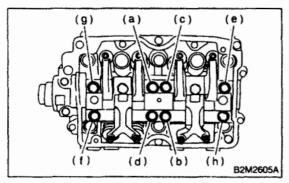
(3) Remove valve rocker assembly.
