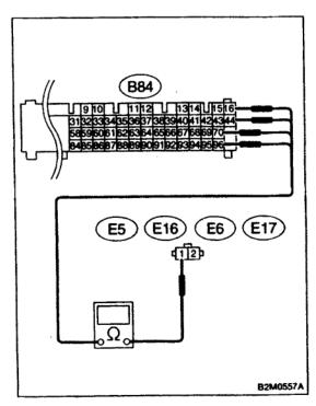
4) Measure resistance of harness connector between ECM connector and fuel injector on faulty cylinders.
