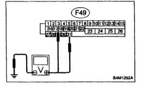
Measure voltage between ABSCM&H/U connector and chassis ground.
