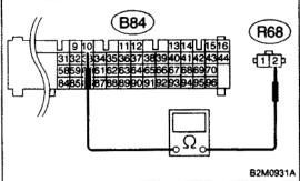
4) Measure resistance of harness between ECM and fuel tank pressure control solenoid valve connector.
