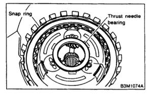
17) Take out retaining plate, drive plate and driven plate of 2-4 brake.
