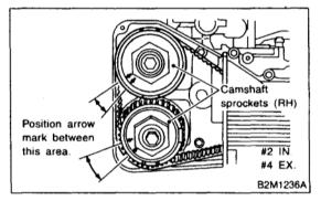
(3) Set arrow mark on camshaft sprocket to position shown in figure, and check #1 cylinder exhaust valve and #4 cylinder intake valve clearances.
