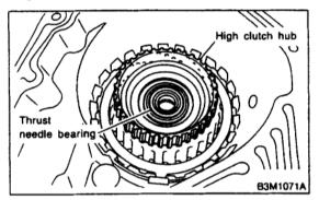
15) Take out the front sun gear and the thrust bearing.
