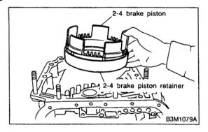
23) Separate 2-4 brake piston and piston retainer.
