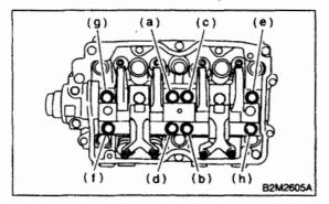
(2) Equally loosen bolts (e) through (h) all the way, being careful that knock pin is not gouged.
