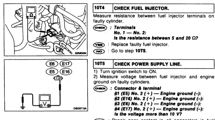
Repair poor contact in all connectors in fuel injector circuit.
