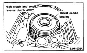
14) Take out the high clutch hub and the thrust bearing.
