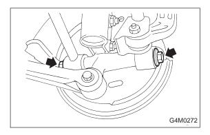
Connect rear spindle assembly to lateral link assembly.
