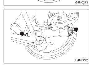
15) Remove bolts which secure lateral link assembly to rear spindle.
