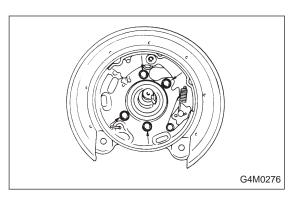
2) Remove back plate from rear spindle.
