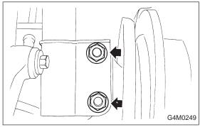
16) Remove bolts which secure strut assembly to rear spindle.
