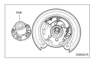
5) Install hub on rear spindle. Temporarily tighten axle nut and washer to hold hub in place.
