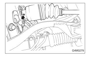
2) Install FTJ on transmission spindle and drive spring pin into place.
