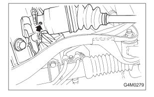
5) Remove spring pin which secures transmission spindle to FTJ.
