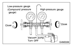
7) Note the low-pressure gauge reading.
