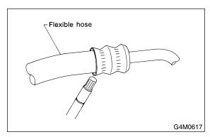
11) Disconnect the drain hose from the evaporator case, and check the hose end for at least 10 seconds.
