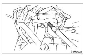
10) Visually check the rubber area of the flexible hose for cracks.
