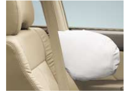
Standard on Outback Limited and Outback H6-3.0 models, front seat side-impact air bags are mounted on the front seats, maintaining optimal placement regardless of seating position. 1
