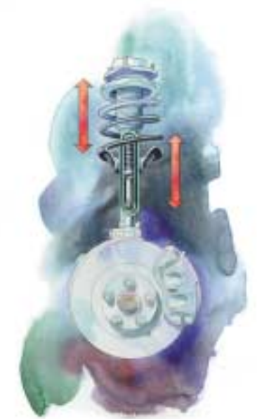
As the body of a vehicle leans in a turn, the suspension of the inside wheel lengthens. All Outback models except Outback Sport feature a rebound spring inside the front strut that is designed to use the mass of the wheels, tires and brakes to resist this lengthening, reducing body roll in turns. The rebound spring also works to reduce the lift of the nose of the vehicle on acceleration.
