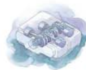
The horizontally opposed boxer design gives a lower center of gravity, which means reduced body roll in turns.
