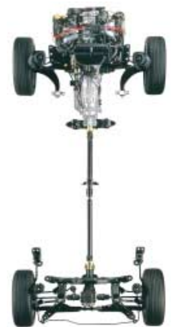
Powertrain components are laid out in a straight line and close to the chassis' centerline, giving agility while providing greater stability.
