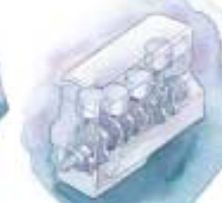
The horizontally opposed boxer design gives a lower center of gravity, which means reduced body roll in turns.
