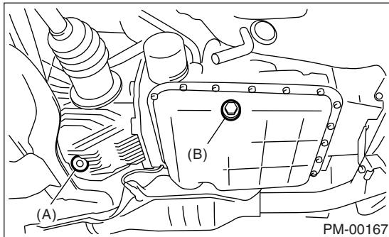
(A) Front differential gear oil drain plug
